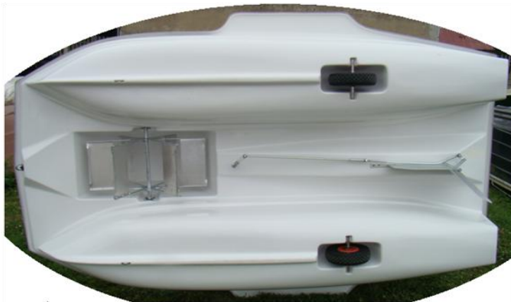
2x wheels under the underwater hull with axles INOX
