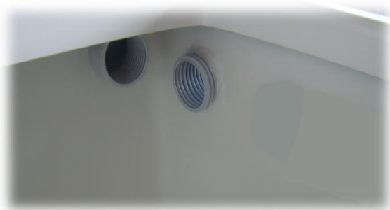
* channels for electric wires between lockers on the left side of the boat
