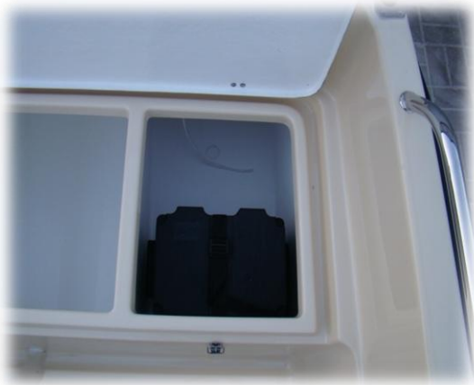
battery box (in the left back locker)
