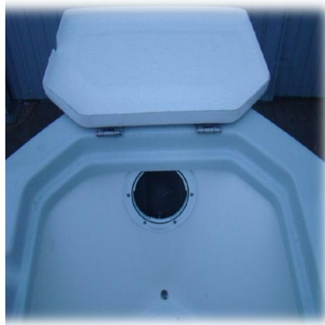
access to montage of the engine on the bow
