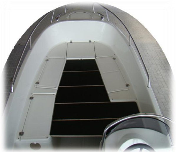
* sun deck / fish deck 5 pieces with waterproof plywood (console to the back)
