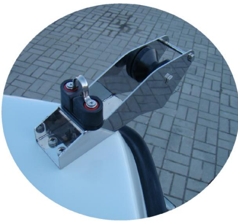
windlass (roll) INOX big with self-clamp and ear INOX
