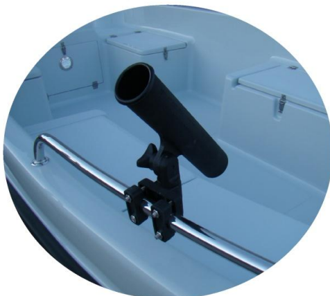
fishing rod socket PCV mounted on the railing
