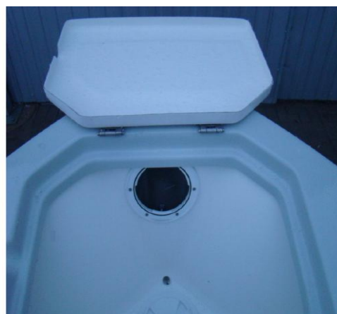
access to the assembly of the engine on the bow
