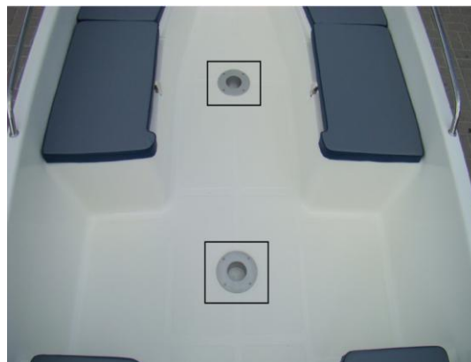
2x sockets for leg of the swivel chair with reinforcement in the floor and montage
