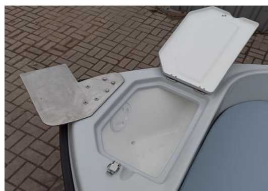
* stand for the electric motor
