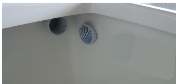
*channels for carring electric wires between lockers on the left side of the boat
