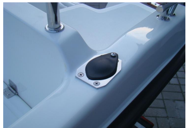
fishing rod socket closed with a plug
