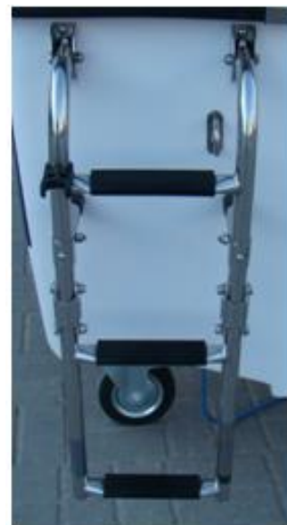
* ladder 3-steps spread INOX, mounted on the left side
