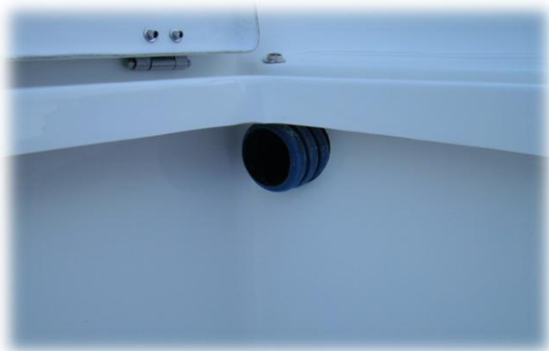
system of channels to put fuel line or electric wires between lockers
