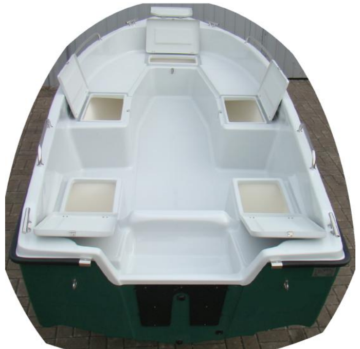
4 lockers at the front of the boat including two (one in the left and one in the right) 130 cm long each
