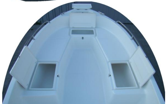
4 lockers at the front of the boat (including 2 at the sides, each one 130 cm long)
