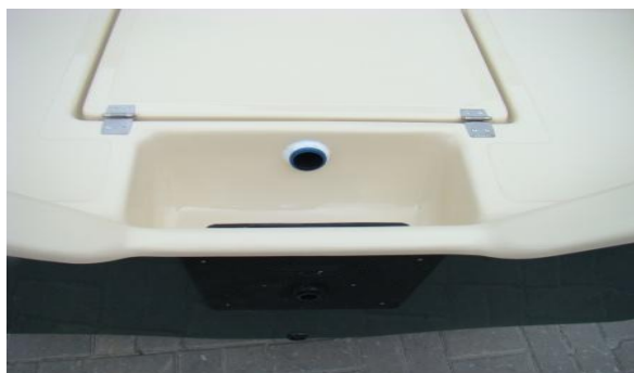
* channel to put wires from engine to the back locker
