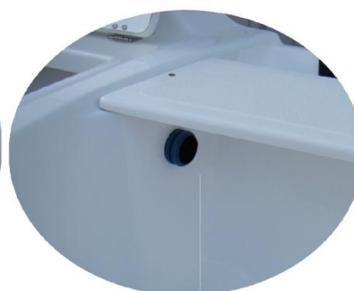
* channel to put wires from engine to the back locker
