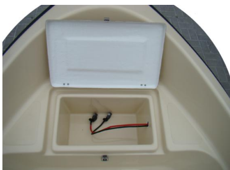
* 2x wires in duct "+" and "-", 2x clamp
