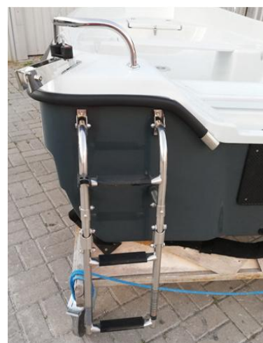
* ladder 3-steps spread INOX, mounted on the left side
