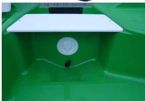
* drain from the deck using the channel
