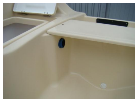
* channel to put wires from engine to the back locker
