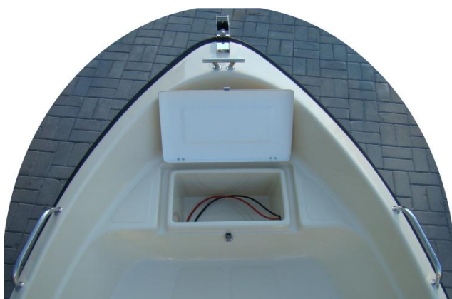
* 2x wires in duct "+" and "-", 2x clamp
