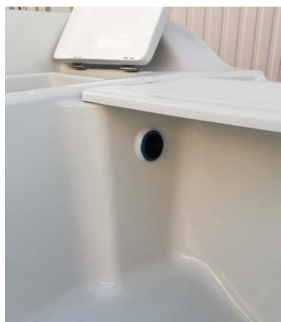
* channel to put wires from engine to the back locker
