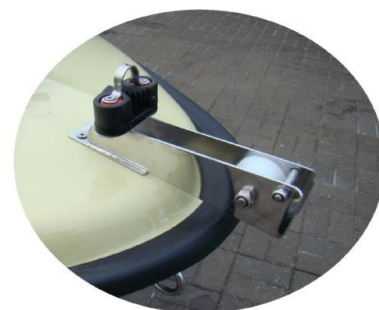
* windlass (roll) INOX smal with self-clamp and ear INOX for weight 5 kg
