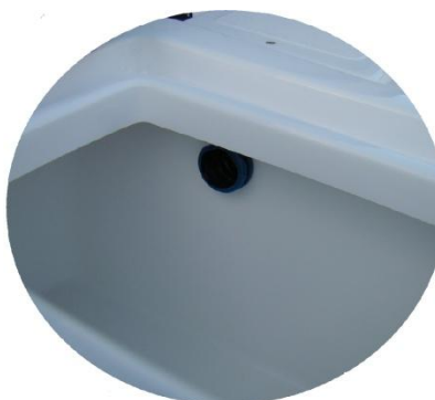
* channel to put wires from engine to the back locker
