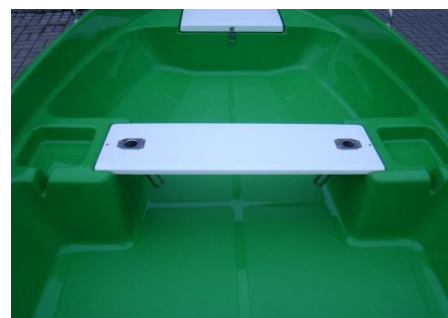
* 2x fishing rod socket INOX mounted in the middle bench
