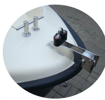
* windlass (roll) INOX smal with self-clamp and ear INOX for weight 5 kg
