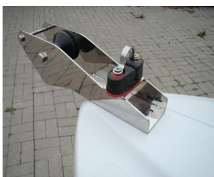
* windlass (roll) INOX big with self-clamp and ear INOX for weight 14 kg
