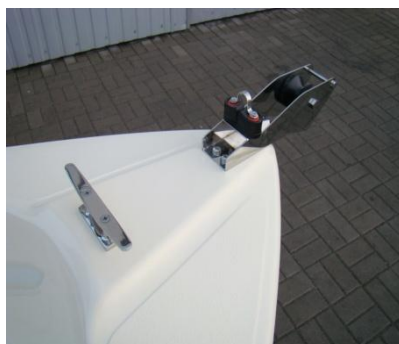
* windlass (roll) INOX big with self-clamp and ear INOX for weight 14 kg
