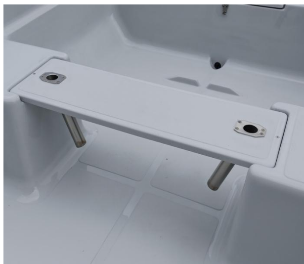
* 2x fishing rod socket INOX available only fishing rod sockets with a plug
